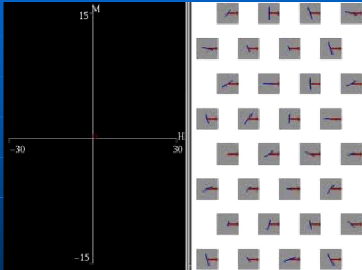
Hysteresis loop in self-assembled FePt nanoparticle array. Movie shows 32 spherical 4 nm particles (though displayed as squares) separated by 6 nm (center-to-center) in hexagonal array,  $H_K=15$  kOe, M vectors in red, easy axes in blue, traces hysteresis loop on MH graph
